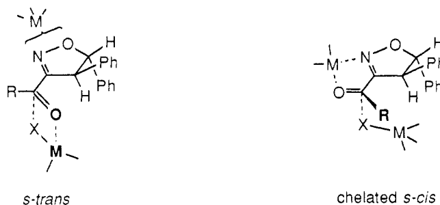
Figure 1. Possible transition states for carbonyl addition and hydride reduction.
